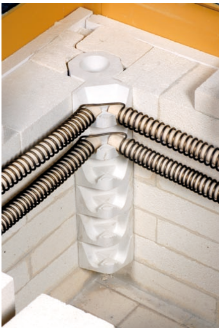
Fig. 13: Enhancement of energy-efficiency, unobstructed radiation from heating elements
